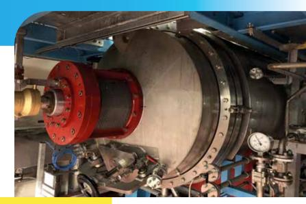
Under moderate operating conditions, dry-running mechanical seals are more robust and service friendly than non-contacting mechanical gas seals. The paddle dryer separates the active substance from the solvent
